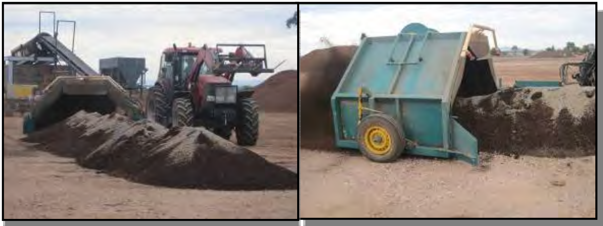
Plate 7 - Mixing seed with humus compost
